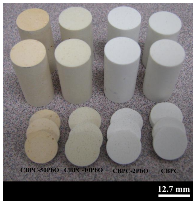
Figure 1 typical irradiation (disks) and compression (cylinders) samples.
